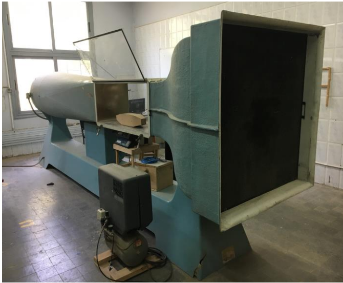
Figure 7 Wind-Tunnel with the basic model in the test section.
