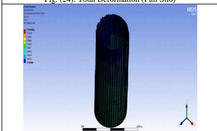
Fig. (25): Equivalent Stress (Full Silo + Wind)
