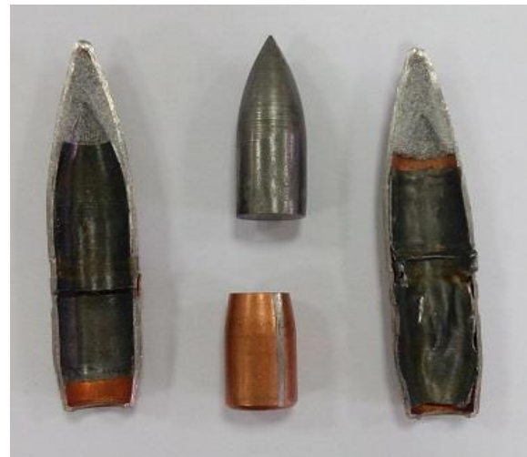
Fig. 1 Shows The Geometry And Composition Of 12.7 Mm Ap Projectile
