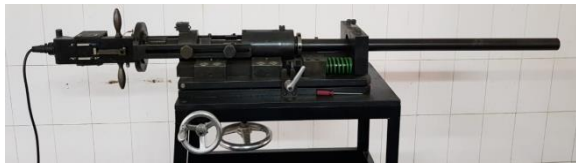
Fig. 12 ballistic barrel used in firing test
