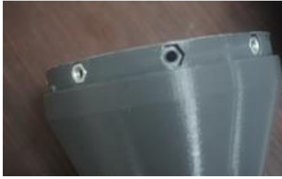
Fig. 12 Connection between parts
