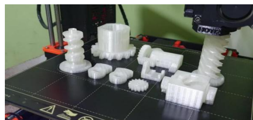
Fig.6 Gears printed with PETG material
