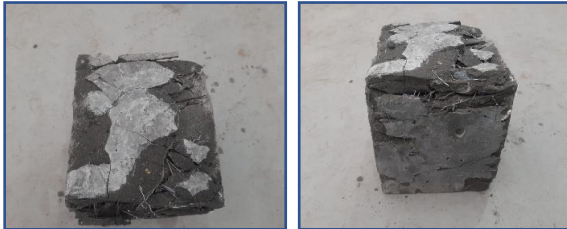
Fig.4 Failure modes of cubes.
