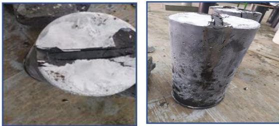
Fig.5. Failure modes of cylinders.
