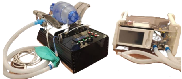
Fig. 18 Both the mechanical and pneumatic ventilators
