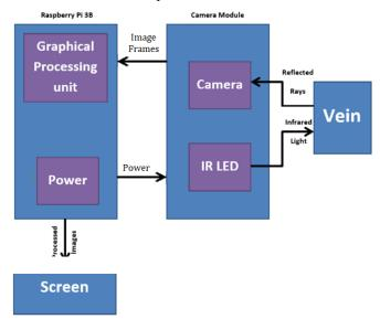
Fig 3 Data/Power Signals Transferred Between the Three Main Layers
