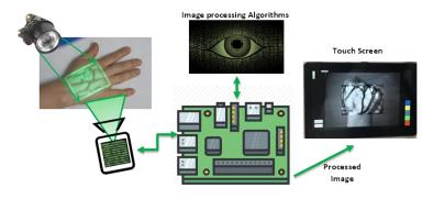
Fig 2 Block Diagram of the Main Layers of Vein Detector
