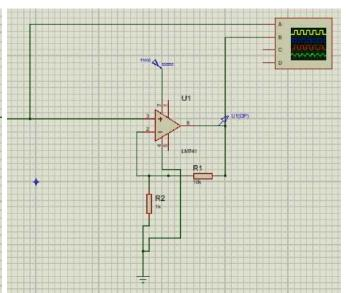
Fig. 4. General schematic of the non-inverting operational amplifier with the gain amplitude with the feedback resistor
