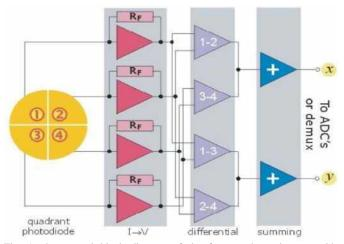
Fig. 1. the general block diagram of the four quadrant detector with processing cicuit for laser position determination/
