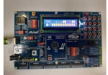
Fig. 10. ADC code by using "Atmel studio " software
