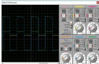
Fig. 5. shows the output of the gain amplifier with the gain amplifier (G=11).
