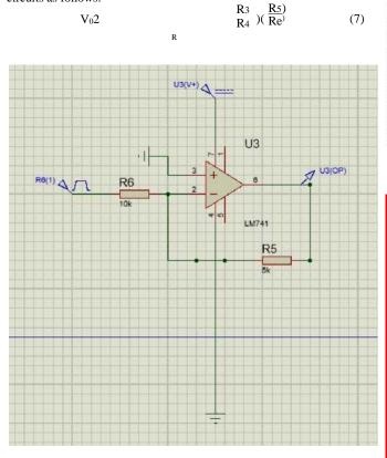
Fig. 7. general schematic of the inverting operational amplifier with the gain amplitude with the feedback resistor  $V_i (1 + \frac{R}{R^2})(1 + \frac{R}{R^2})$
