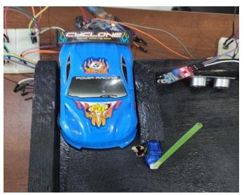
Fig 2 Car detected by IR sensor when entering the gate
