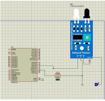
Fig 3 IR sensor and Servo motor connections for the automated gate
