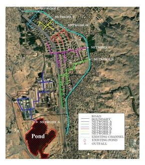
Fig. 20: Storm Network for Zone A
