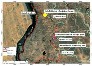
Fig. 18 Conceptual Design of Alternative 02
