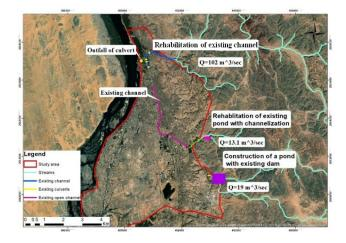
Fig. 17 Conceptual Design for Alternative 01
