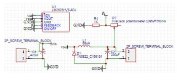
Figure 12 LM2576T-Adj schematic
