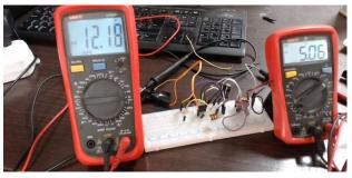
Figure 13 LM2576T-Adj implemented in breadboard
