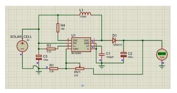
Figure 10 Simulation of boost converter
