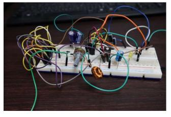
Figure 11 Boost converter implemented in breadboard
