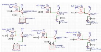
Figure 15 Switching circuit schematic
