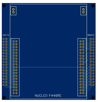
Figure 23 Secondary PCB contains STM 2D
