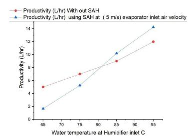
Fig. 2 Effect of using Solar Air Heater (SAH) on Unit Productivity
