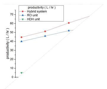
HDH unit and RO unit individually. The maximum productivity is about 70 L/hr. which has increased by 550 percentage difference than HDH unit productivity and 39 percentage difference than RO unit at 95 C water temperature at humidifier inlet
