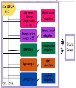
Figure IV (CubeSat lite OBC Architecture)
