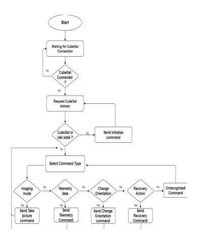
Figure IV.VII (Software Code Flowchart)
