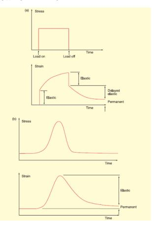
Fig. (5) Visco-elastic responses of a sphalt under (a) a static load and (b) a moving wheel load
