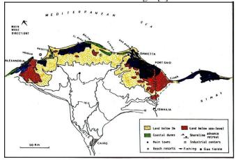
Figure 1 General Topography Of The Nile Delta Indicating Areas Below Mean Sea Level In Red And Areas Below 2m Contour Level In Yellow (El Raey, 2010).
