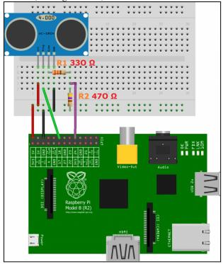
Fig. 6 Schematic diagram of Ultrasonic sensor with Raspberry pi 3.
