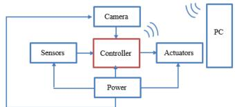
Fig. 3 Generic block diagram of the self-driving car.
