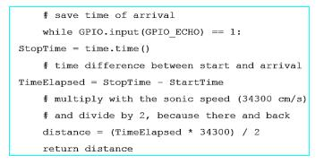
Fig.7 Part of ultrasonic sensor using python code.
