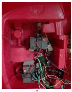
Fig. 5: Parts of hardware components inside the self-driving car prototype (a) front ultrasonic sensors, (b) Batteries and Raspberry pi 3 module.
