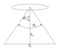
Figure 7: The camera angle of view
